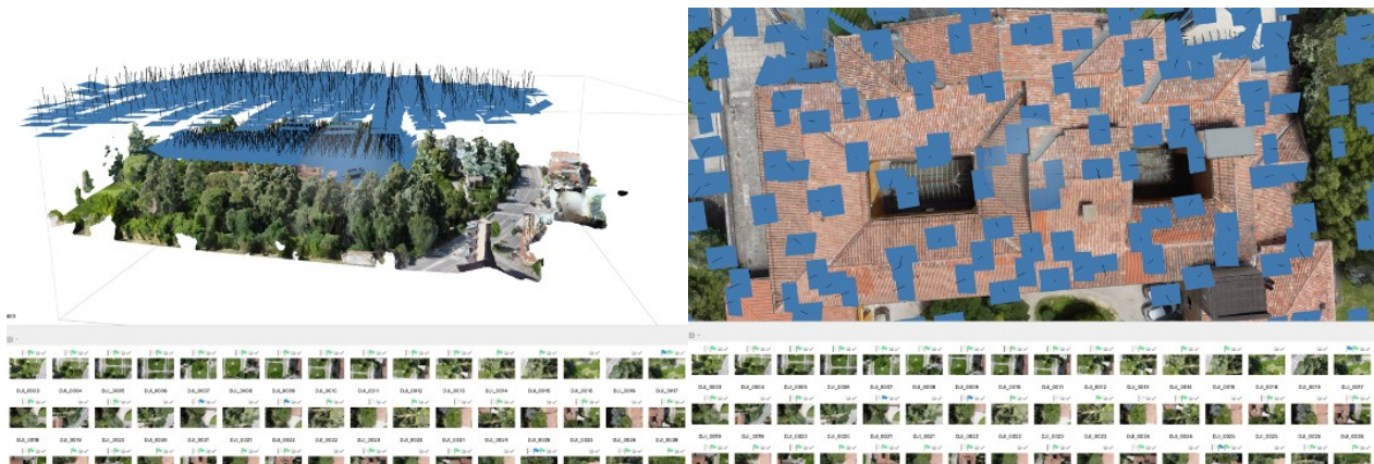
Figure 64. Textured mesh from photogrammetry with estimated picture positions of the exterior and the surroundings of the Villa (left) and a detail highlighting the pattern of the pictures (right)
