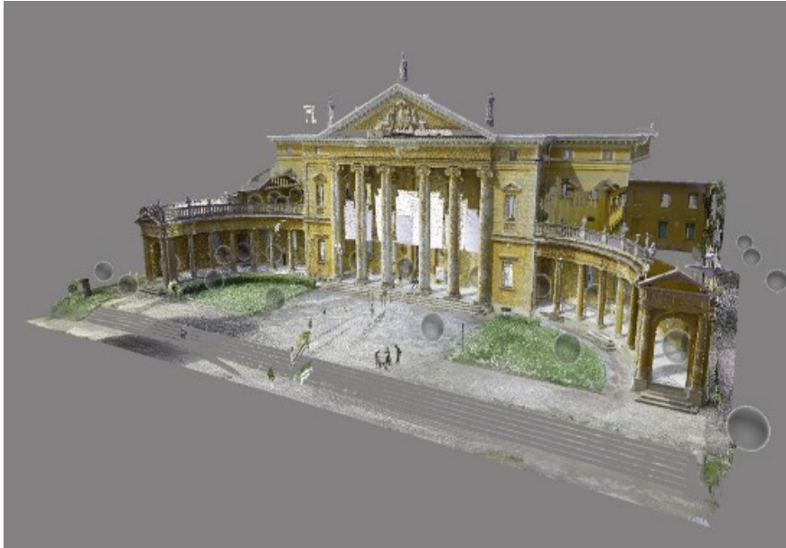
Figure 60. Point cloud from TLS with bubbles representing the scanning positions
