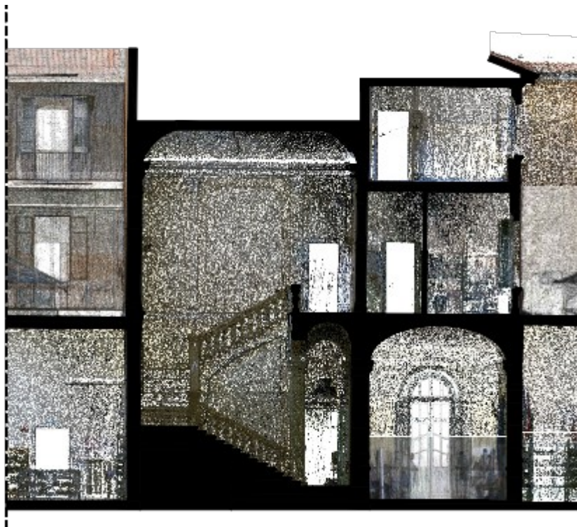
Figure 67. CAD drawing of the Grand Staircase of the Villa based on the overall point cloud (scanner + photogrammetry)
