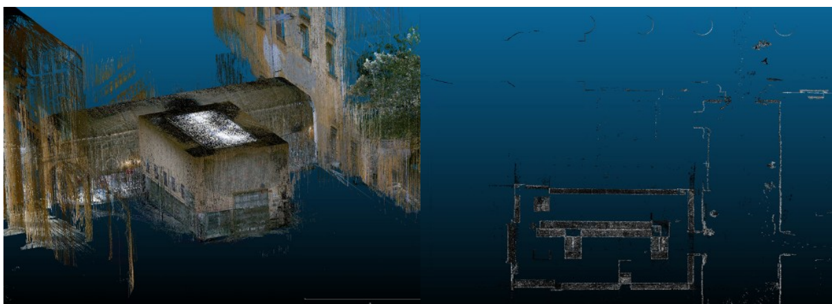
Figure 63. Point cloud from the Leica BLK2GO in perspective view (left) and top view, with a bounding box extrapolating a horizontal slice of 10cm (right)
