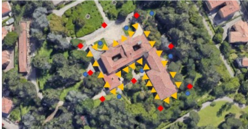
Figure 59. Schema of target positions for the exteriors (blu dots: targets for aerial photogrammetry; red squares: TPS positions; yellow triangles: targets for TLS and ground photogrammetry)
